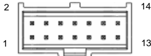
OEM module: Top view, 14 pin header Connector Type: Molex (C-Grid III), dual row
