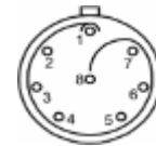
Shielded Remote module: Looking into connector Connector Type: Lemo 1B 8-pole
